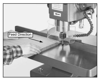
Figure 26. Straight routing direction.
